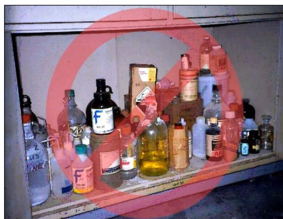
**Figure VI-I. Improper Fume Hood Storage**
